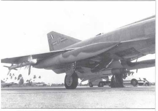
First RAAF Mirage to be loaded with Matra "Magic" Missile. Standard Matra Missile fitted under centre fuselage.
