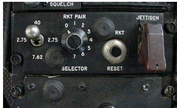
'Bushranger' gunship Weapon Select Panel – 2.75 inch rockets HE x six, single fire or pairs; WP x one, single fire for target marking.
