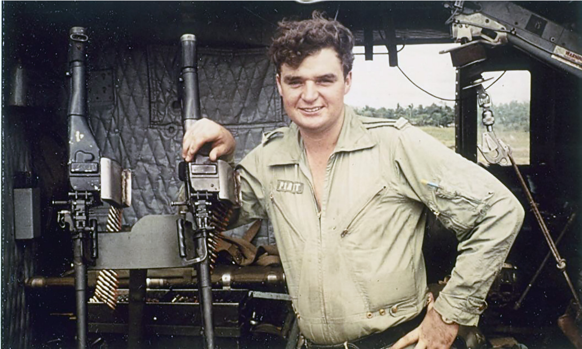
Above: Nev Pratt, ADG and No 9 SQN RAAF gunner, pictured at twin starboard M60 machine gun station during a mission to Cambodia in late Nov 70 - see pages 98 & 99, Detachment to Phnom Penh. Twin machine guns were fitted to the three Huey slicks on that mission. Normally slicks were fitted with one machine gun per side.
