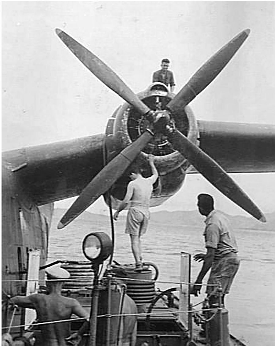
Port Moresby, Dutch New Guinea. 1944-09-21. A Papuan native (right) assists to refuel a Martin PBM Mariner flying boat aircraft of No. 41 (Transport Sea) Squadron RAAF based at Cairns, from a refuelling barge.
