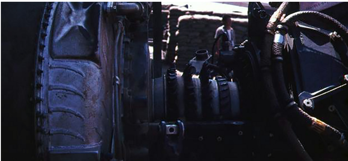
Below: Engine compressor damage/failure of Iroquois A2-1022 that occurred on 11 May 1967.
